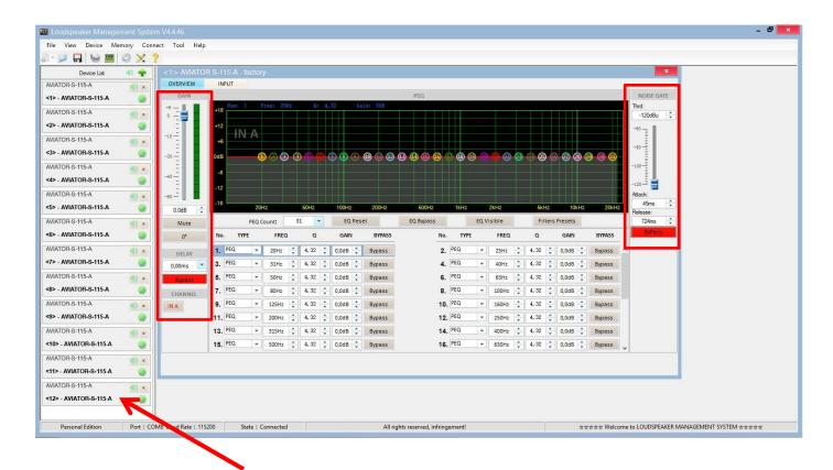
To apply changes to any of the units connected to the ProDGnet network, simply click on the desired unit.
