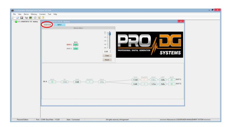
This menu allows modifying different options on input A and outputs 1 and 2, such as: Mute, Limiter, Gain, Polarity and Delay.
